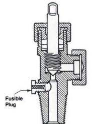
Figure 2. Sulfur Dioxide Header Valve
