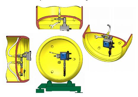
AW—Actuator Mounting Ton Ironworks Ironworks has YAH-319 eccentric extender added for use with emergency shutoff actuators.
