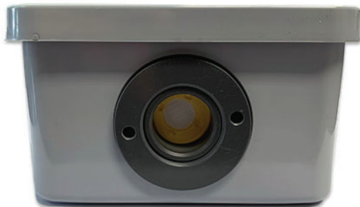
FIGURE 2a Exposed Gas Sensor
